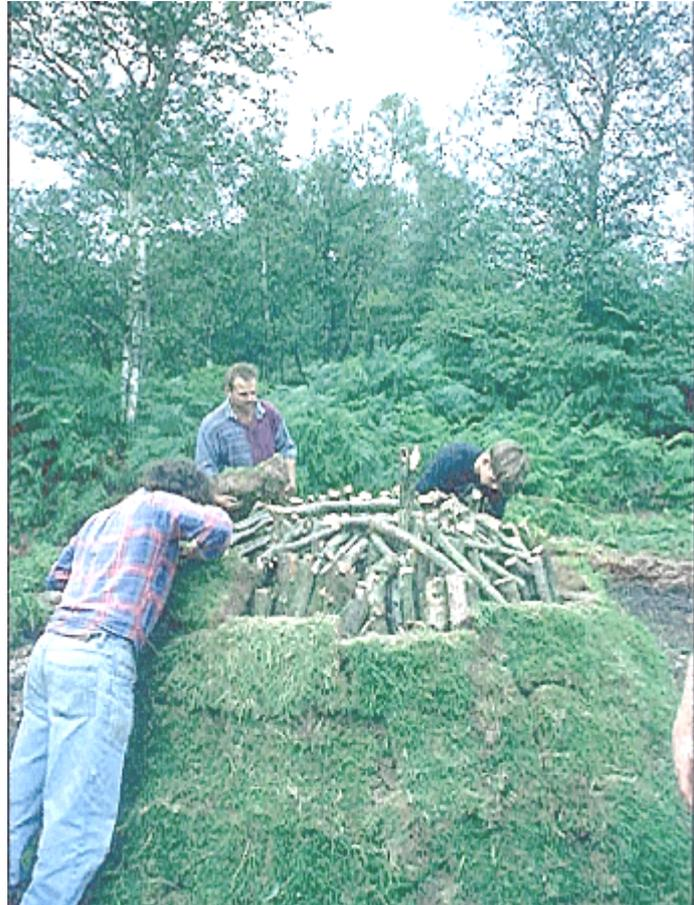
Construction of a Traditional earth covered Charcoal making Clamp
